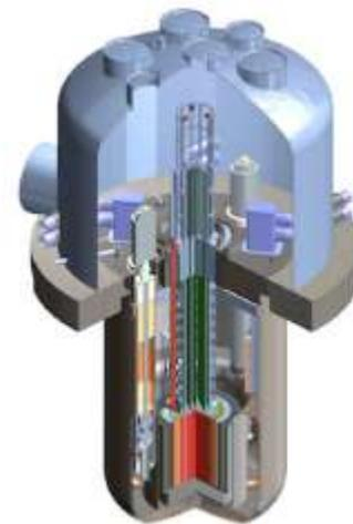
Turns depleted uranium into electricity, using a simple fuel cycle without requiring separations.
